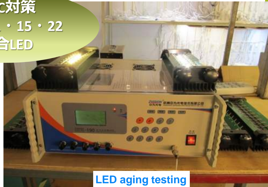
LED aging testing
