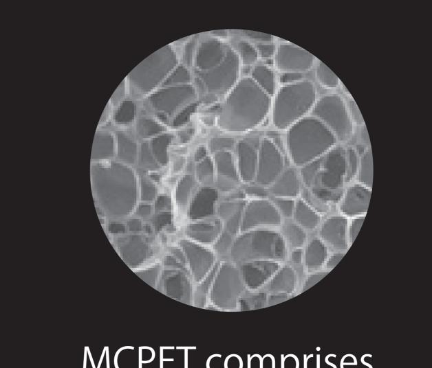
MCPET comprises the closed-cell foam element
