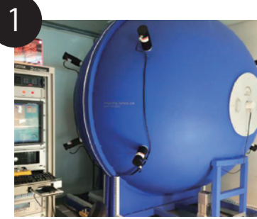
Integrating Sphere Test
